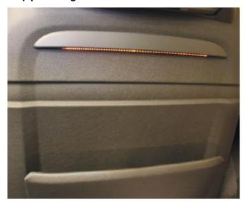
**Sill Lights**The sill lights are connected directly to the footwell module. LEDs are used as the light source. All four doors have sill lights.
